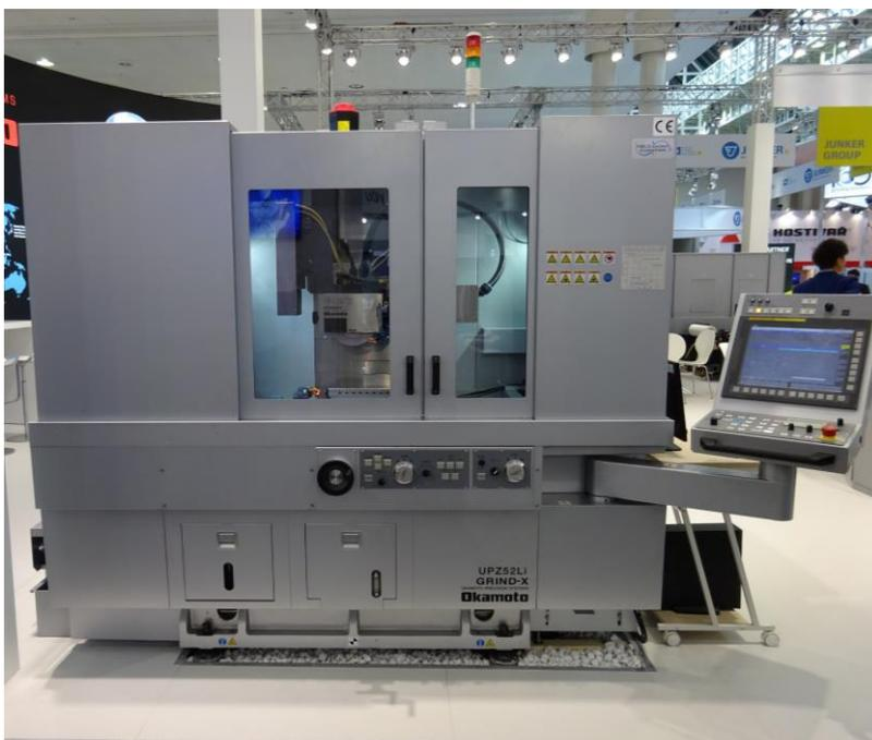
A linear motor drive achieves in 500+ reciprocations /min over a 10mm stroke with a stroke reversal accuracy down to 1 micron. Coupled with a small constant down feed, this oscillation speed drastically increases productivity.
