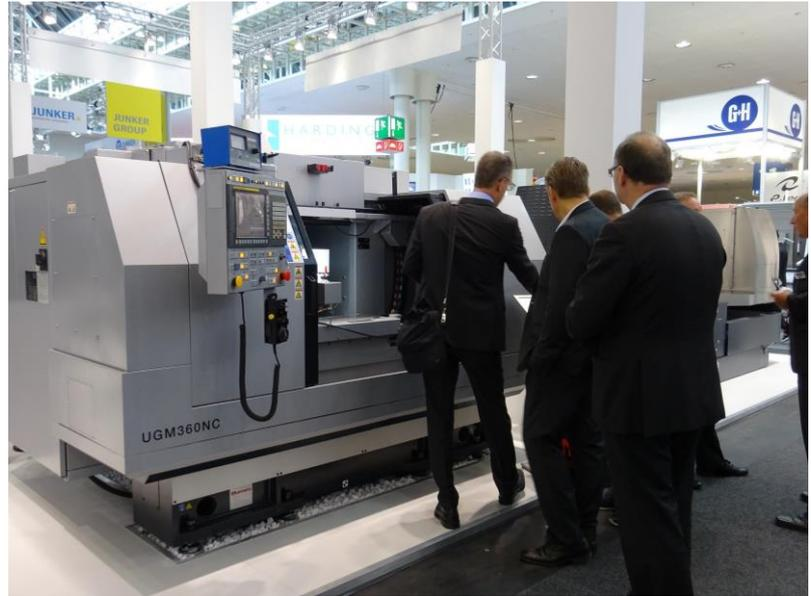
turret. All grinding wheels are mounted on self contained, self driven high frequency type spindles with built in thermal cooling. Two external wheels with  $\varnothing 500\text{mm}$  may be mounted on the same turret in addition to the internal spindle. A range of self driven internal spindles is offered from 10,000 r.p.m. up to 60,000 r.p.m. and beyond.
